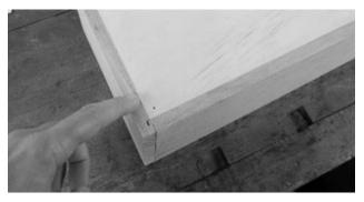
Clamp box as shown and wipe off excess glue. Check assembly for squareness with 90-degree square. Allow time for glue to dry before handling and double check to make sure the bottom is flush with the frame components.
