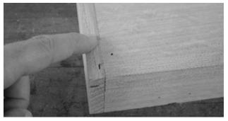
Glue and clamp in the same way that the bottom section was completed in Step 3. Remove excess glue and check top for square.
