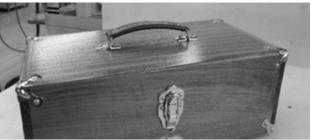
Install the Gerstner nameplate where desired. We typically place the nameplate on the front for this style of chest. After installation, remove the protective film to expose the beauty and luster of the nameplate.
