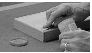
Sand the surfaces flush using your preferred method. An orbital sander will greatly reduce the amount of work required. We sand chests with 120-150 grit paper before applying the stain and finish. USE CAUTION when sanding the top veneer, as it is very thin and can be damaged easily!
